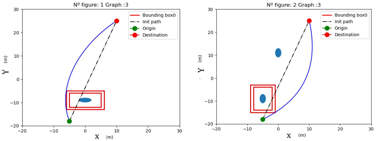
Figure 5: Left: Execution of the algorithm with 1 obstacle. Right: Execution of the algorithm with 2 obstacles.
